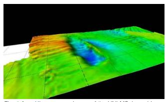
Fig. 1 A multibeam sonar image of the HNLMS Java shipwreck location that is clearly showing the hole in the seabed where once the ship was lying. © KDF/Royal Dutch Navy.
