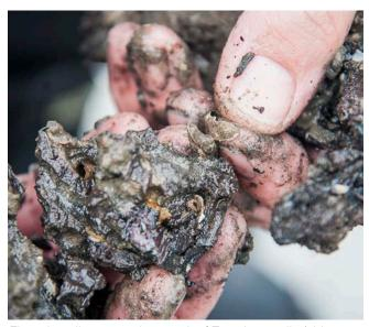
Fig. 1 In saline water the attack of Teredo navalis (shipworm) is an enormous threat to shipwrecks and other wooden structures. Here we can see the devastating effect the shipworm has on historical shipwrecks. The wood has crumbled and almost disappeared. © Paul Voorthuis, High Zone Photography.
