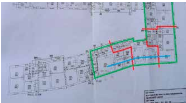
Fig. 3 Plan of a historic building in the town centre after the nationalisation of the private property, showing the division of the apartments into social flats
